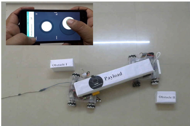
Fig. 9 An operator remotely maneuvering using two analog joysticks(left for orientation and right for translation control) the leader robot through the obstacles as per visual feedback
